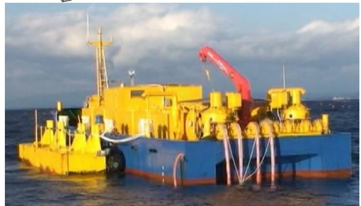
Feeding barge that can withstand the significant wave heights of less than 4m
