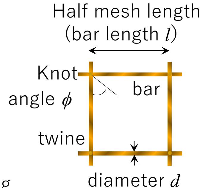
$\rho$  (kg/m<sup>3</sup>): water density  $C_D$  (-): drag coefficient
